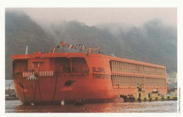
Using its float-on/float-off technique, Crowley loaded this entire dredge fleet onto a single barge for transportation from the U.S. to Kenya.
