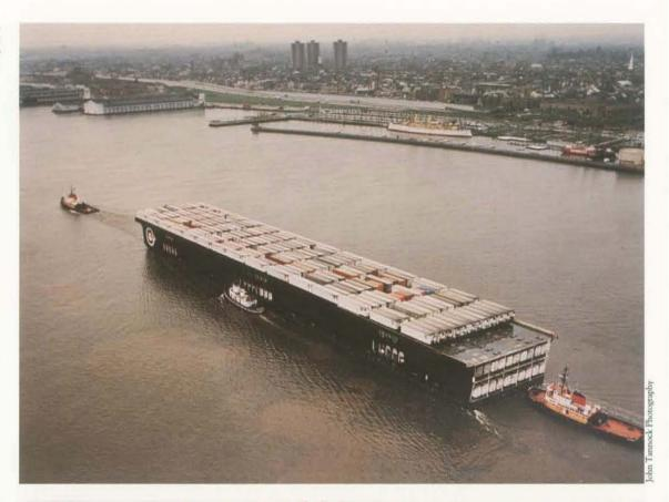
Trailers are loaded or offloaded on all three decks of a triple-deck barge simultaneously by means of triple-deck ramps at all company terminals serving the mainland/Puerto Rico trade route. Shown is the Northeast terminal, a 58-acre site at Pennsauken, New Jersey, near Philadelphia.
