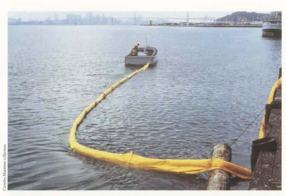
A CES workboat deploys oil spill containment boom.
