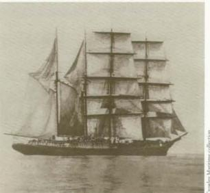
$Left, the five-masted schooner\ Crowley\ was\ built\ from\ a\ raised\ coal\ barge,\ the\ ex-City\ of\ Panama,\ and\ used\ to\ carry\ cargo\ to\ Australia\ during\ World\ War\ 1.\ Right,\ the\ one-of-a-kind\ barkentine\ Olympic\ was\ used\ in\ ocean\ and\ coastal\ transports.\ (These\ images\ were\ processed\ from\ original\ daguerreotypes.)$
