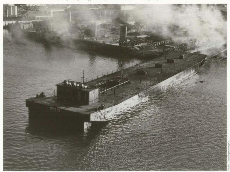
Numerous bulk petroleum barges were added to the Crowley fleet in the 1950s to keep pace with the company's growing involvement in petroleum transportation. Barge 50 came off the ways in 1953 at Pacific Coast Engineering Company. The 260 x 48 x 12-ft. barge had a capacity of 24,224 barrels.
