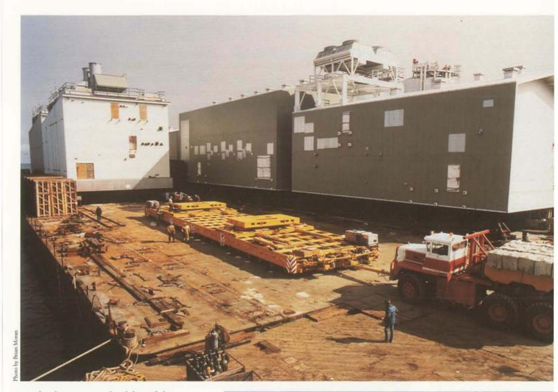
overland transports of sealift modules. Shaughnessy provides heavy-hauling, rigging, and millwright services throughout the western United States and Alaska. Today, its trailer fleet includes rubber-tired, hydraulic platform trailers (RTVs) that can haul modular units up to 3,200 tons and can be configured with as many axles as are needed for the cargo.
