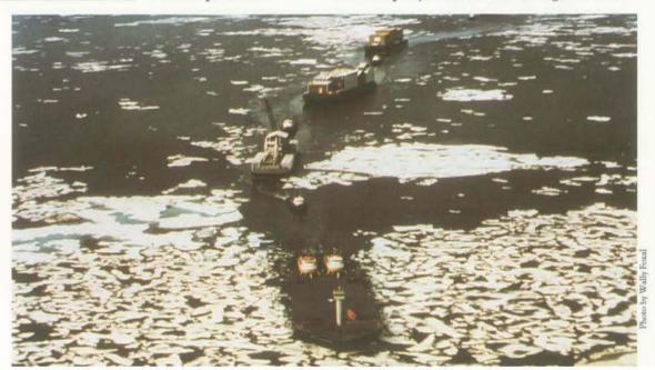
Crowley's icebreaker barge Arctic Challenger, pushed by two 9,000h.p. tugs, opens a path through the ice for the 1976 sealift fleet.
