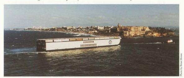
A second deck added to TMT's 400-ft. trailer barges doubled their capacity to 180 trailers each.
