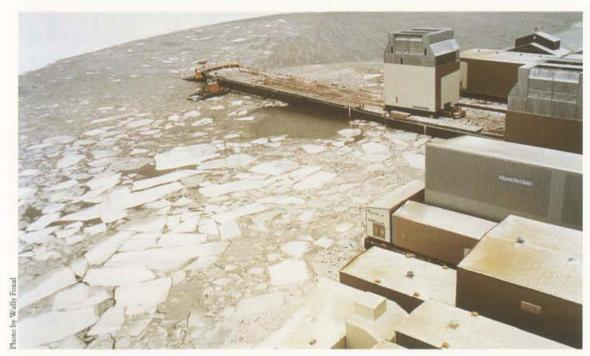
The 1975 sealift module barges were stopped by ice within a mile of the discharge site. Some modules were lightered to the dock, but most remained offshore on barges frozen in place until the oil companies extended a gravel causeway from the dock to the captive vessels.
