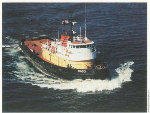
triple rudders. Outfitted with double-drum towing winches, they are used to tow the company's large oceangoing barges either singly or in tandem.
