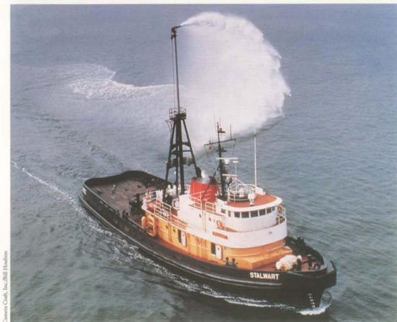
The 9,000-h.p. tug Stalwart demonstrates some of its firefighting capability. Assigned to Valdez Harbor, the tug is specially equipped to perform rescue towing, as well as tanker docking and escort services. every regulatory requirement in a thoughtful and comprehensive manner..."
