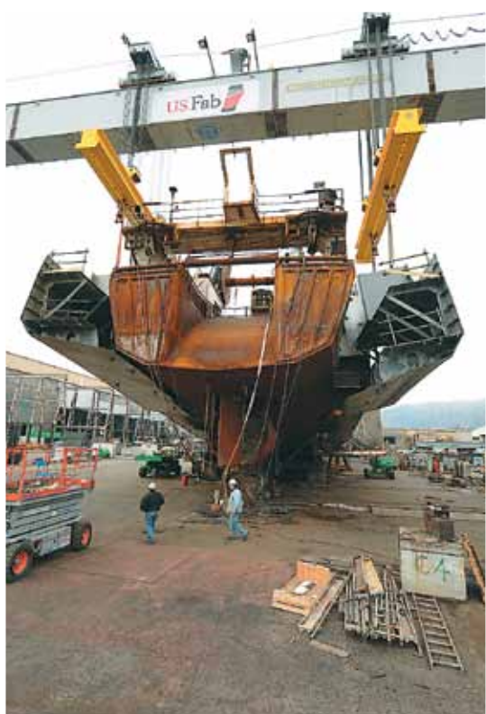
Vigor Marine's Portland, Ore., crew hauled out the 28-year-old, 220-foot Ocean Peace for a sponsoring job. She also got a rebuilt bow with a bulb.
