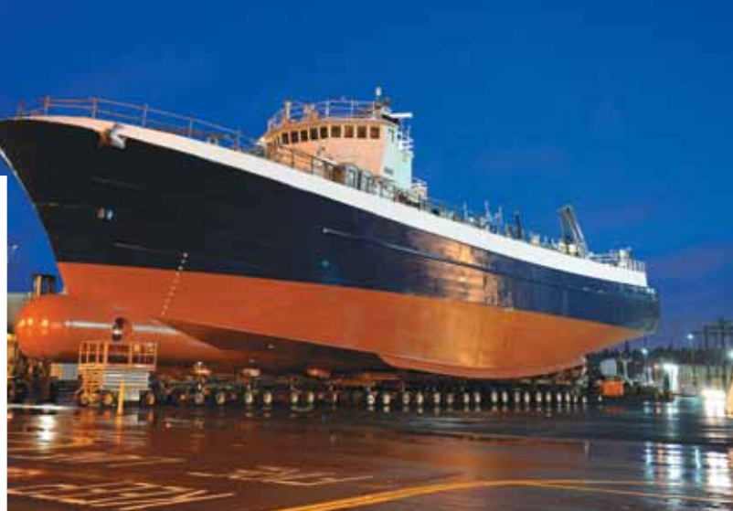
Vigor Marine's Portland, Ore., crew hauled out the 28-year-old, 220-foot Ocean Peace for a sponsoring job. She also got a rebuilt bow with a bulb.
