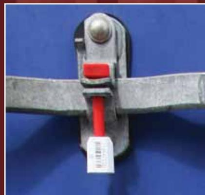
*Special round-headed huck bolts are used on all door-mounted hardware.*
