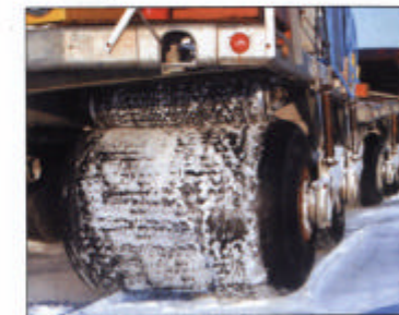
CATCOs have eight wheels, 10 if the trailer is being used. Each wheel is independently powered by a roller, which sets on top of the tire. Traction is achieved by the weight of the cargo deck and its payload.
