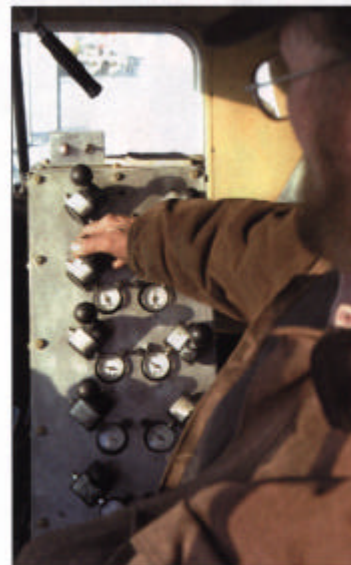
Ron Hansel demonstrates the 10-knobs operating system that manages the air pressure for each tire. Tire pressure can be independently controlled, and it can be done while the CATCO is moving.
