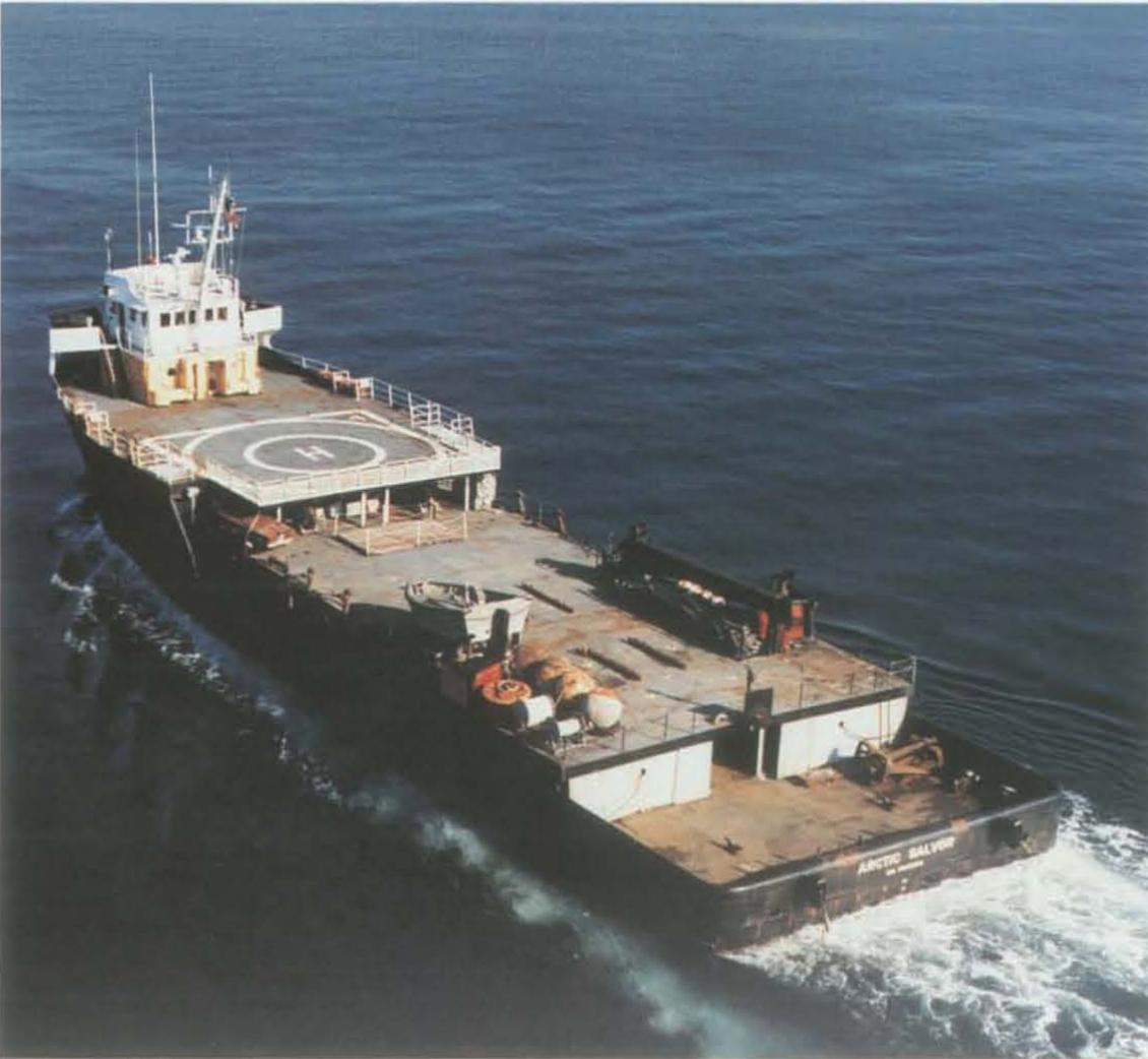
The Arctic Salvor is outfitted for all types of heavy-duty marine salvage work, including wreck removal, raising sunken vessels, underwater repairs, and refloating grounded ships.
