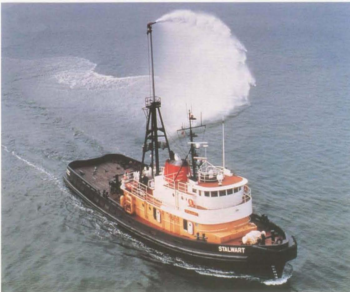
The 9,000-h.p. tug Stalwart demonstrates some of its firefighting capability. Assigned to Valdez Harbor, the tug is specially equipped to perform rescue towing, as well as tanker docking and escort services.
