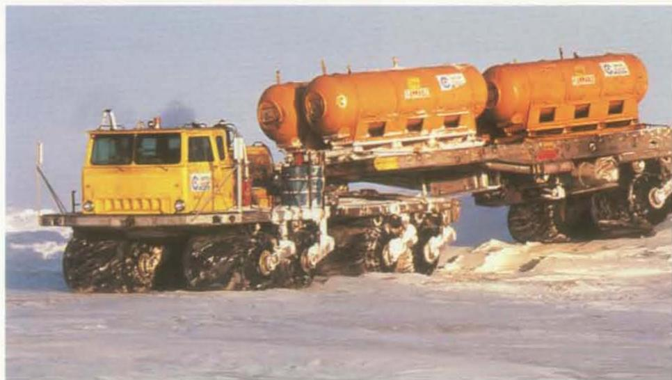
Top, Shaughnessy & Company's rubber-tired trailers are used to offload modules from barges at Prudhoe Bay and transport them inland.
