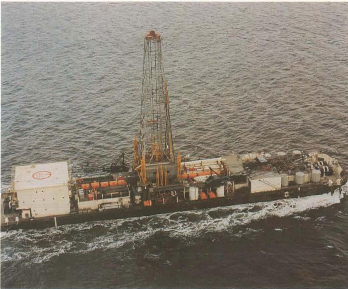
The 400-ft. drill barge Brinkerhoff I is capable of drilling to 20,000 feet into the ocean floor.
