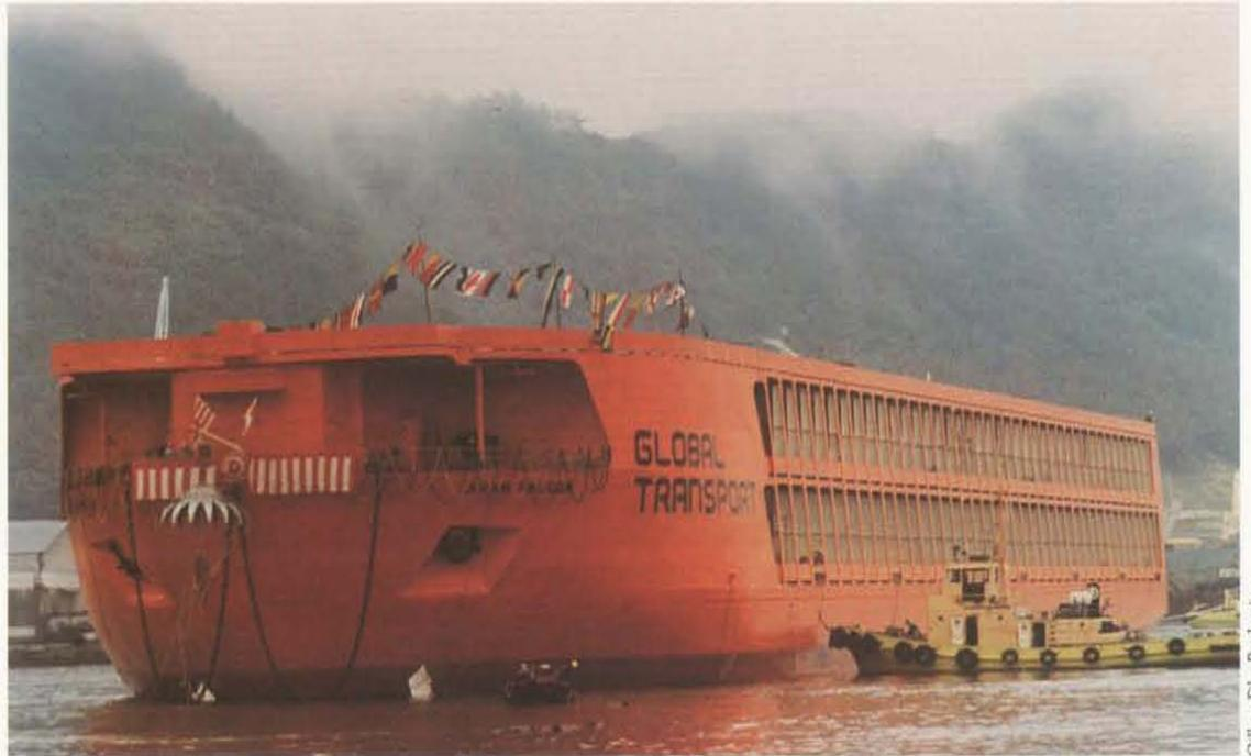
Using its float-on/float-off technique, Crowley loaded this entire dredge fleet onto a single barge for transportation from the U.S. to Kenya.
