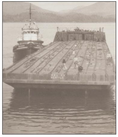
Barge ABC 20, used in the 1950s, was equipped to transport railcars between Ketchikan, AK, and Prince Rupert, British Columbia, Canada.
