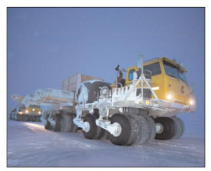
CATCO all-terrain vehicles were first acquired in 1975 for remote off-road transportation in support of the oil industry.
